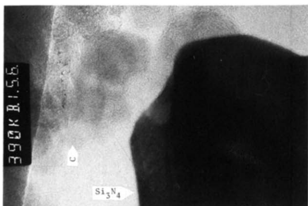
Fig. 5. The mixture at 55% conversion. The length of the black bar is 130 nm. Gas black particles with a diameter of 35 nm and a crystalline \text{Si}_3\text{N}_4 particle are shown.
